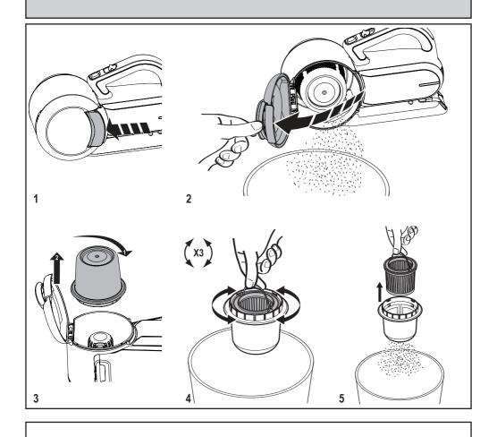
Re-assemble after cleaning the filter or continue to wash.
